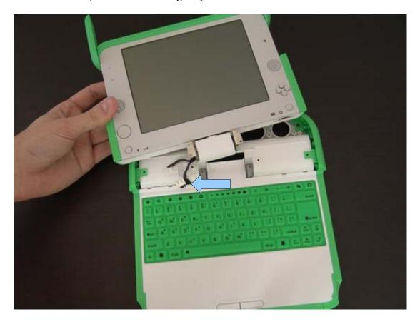
Disconnect the power cable marked above with the blue arrow.
