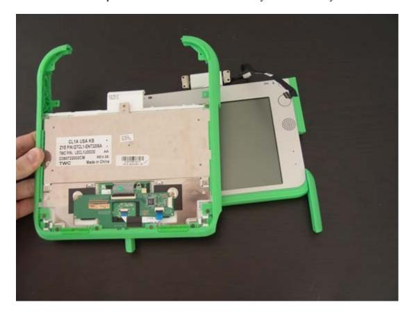
To further disassemble the keyboard. Remove the 8 screws that hold the green edges. And the 4 screw holding the keyboard in place.
