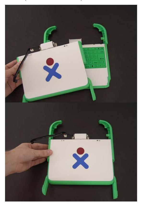
Flip the unit over again and re-attach the keyboard and touch pad cable.
