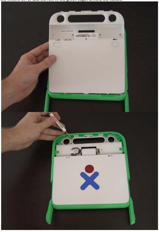
Flip the unit one more time and secure the LCD screen bracket with the four screws.
