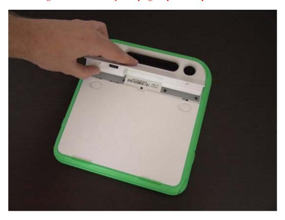
Undo the five screws from the bottom of the battery compartment.
