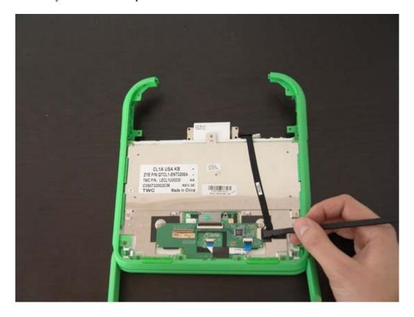
You should now be able to separate the LCD screen from the keyboard assembly.
