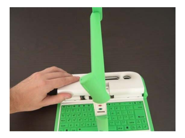
Remove the 4 screws that hold the green side edges of the laptop.
