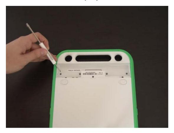
Flip the laptop over and rotate the screen 90° in either direction. You should now be able to remove the top panel by gently prying it up.
